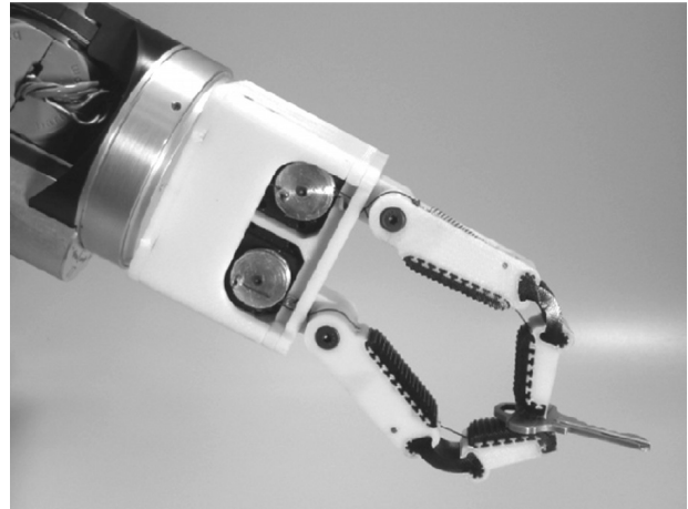
Fig. 1. A thin object, such as a key, must often be reoriented during the grasp acquisition process. Consequently, in-hand manipulation is critical to the operation of any dexterous robot hand.
