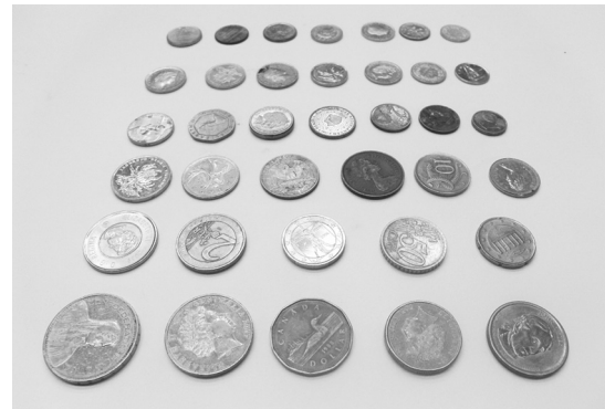
Fig. 10. An array of coins, denominated in AUD, EU, CAD, CHF, RMB, and USD were used as test objects to determine the range of width and thickness graspable with the hand.
