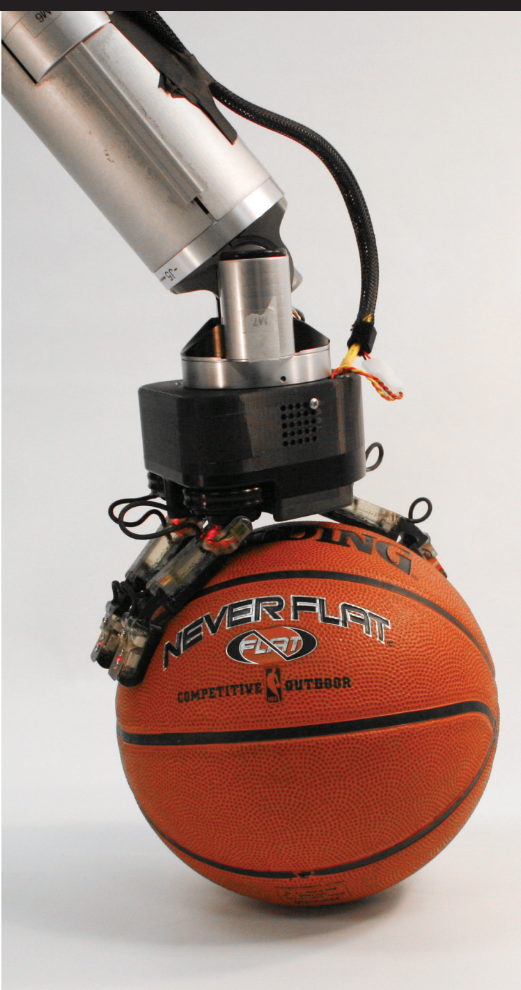
STARTING FROM SCRATCH: To develop a robotic gripper that can handle objects large and small, researchers at Harvard, Yale, and iRobot abandoned the familiar human hand, aiming to re-create its functions with a simpler design.
