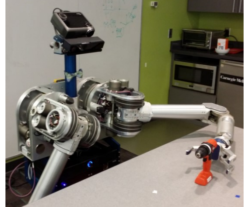
Fig. 10: (left) Screen-capture from Openrave simulation and planning environment showing the HERB robot planning a grasp of the power drill object in the set. (right) actual grasp being executed by the robot on the physical object.
