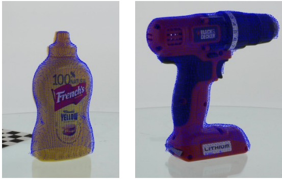
Fig. 9: Point cloud and textural data overlays on two YCB objects: mustard bottle and power drill.
