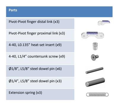
Install the 4-40 inserts for the distal joint spring and the distal tendon anchor. You can alternatively thread a bolt directly into the specified points. An extension spring or elastic band should be anchored on bolts threaded into the inserts closest to the distal joint.
