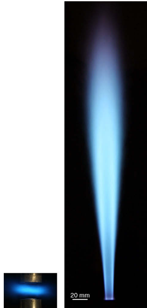
Fig. 10. Long-exposure photograph of \text{C}_2\text{H}_4 non-premixed flames at comparable cold Re_t \sim 10^3 and Re_0 \sim 10^4 in counterflow (left) and co-flow (right) configurations. Both photographs are reproduced in the same scale.
