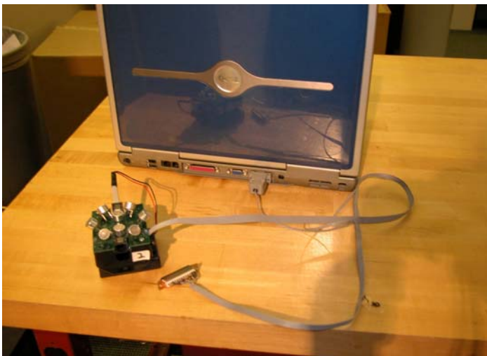
Figure 6 PC node connect with Laptop
