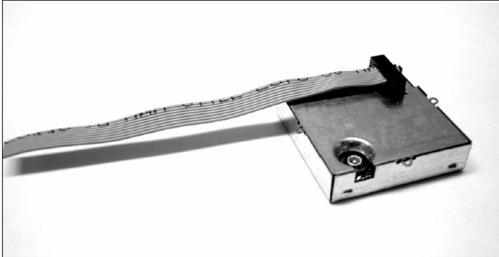
Figure 2 FFSD connector mount on GPS Receiver
