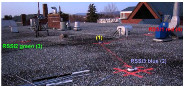
Figure 3. Rooftop Deployment scenario. Center receive node is at position 1. Transmit nodes are each 6m from the center.
