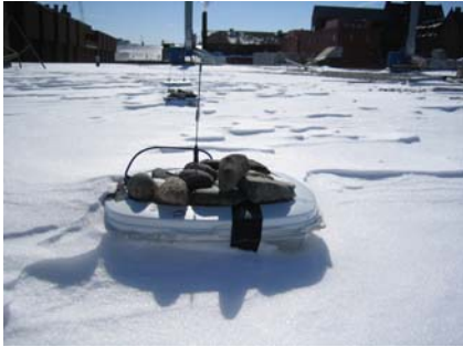
Figure 2. Chipcon evaluation board deployed in weatherproof enclosure on the roof at UVM.
